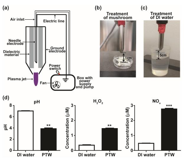
**Figure 1.** Treatment with NTAPPJ (non-thermal atmospheric pressure plasma jet) and properties of PTW (plasma-treated water). (a) Schematic view of NTAPPJ device. (b) Photo of treatment of mushroom pieces with NTAPPJ. (c) Photo of treatment of deionized water with NTAPPJ. (d) pH of PTW and level of  $H_2O_2$  and  $NO_x$  measured in PTW. Each value is the average of nine replicate measurements. \*\* p < 0.01, \*\*\* p < 0.001.
