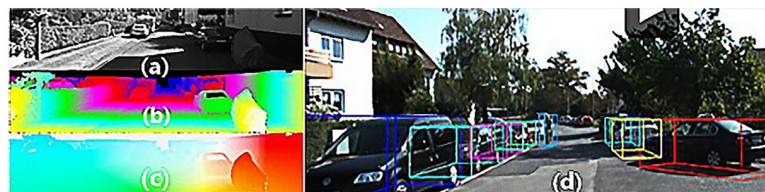
Fig 2. The depths and stereo images of the datasets. (a) shows an RGB image. (b) and (c) show different depths of LiDAR scanning images. (d) shows a 3D labeled image in the perspective of the camera.
