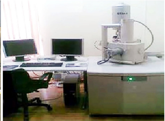
Figure 4 – The Inspect S device used for SEM/EDX analysis. SEM/EDX: Scanning electron microscopy/ Energy-dispersive X-ray.
