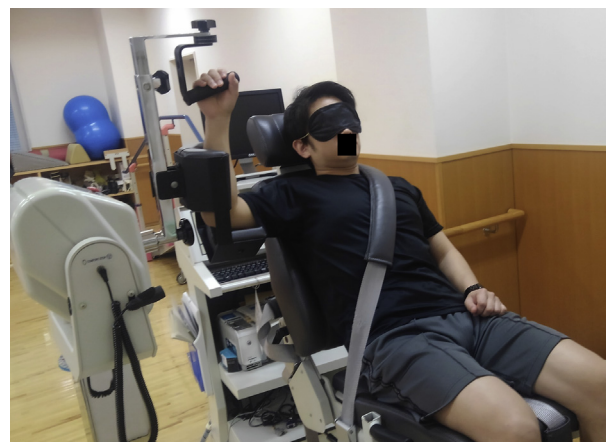
Figure 1 Measurement of position sense using the Biodex System 3. The trunk of the patient was fixed with a seat belt and the patient was blindfolded to prevent visual assistance.
