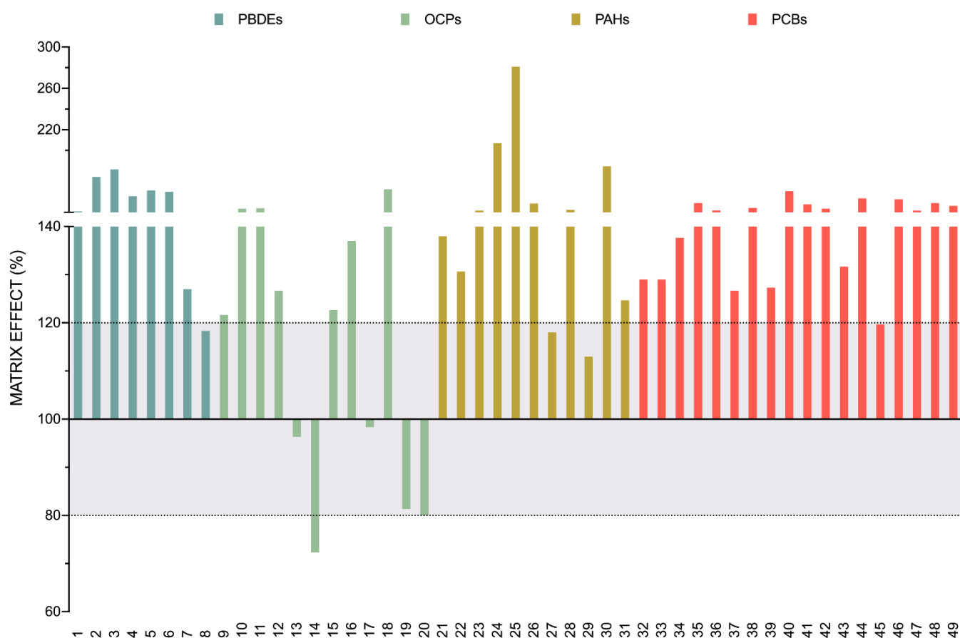
Figure 3. Matrix effect. Bars represent the mean of the ME% of the analytes. Dotted lines represent the tolerance range in which it is considered that no significant matrix effect exists.
