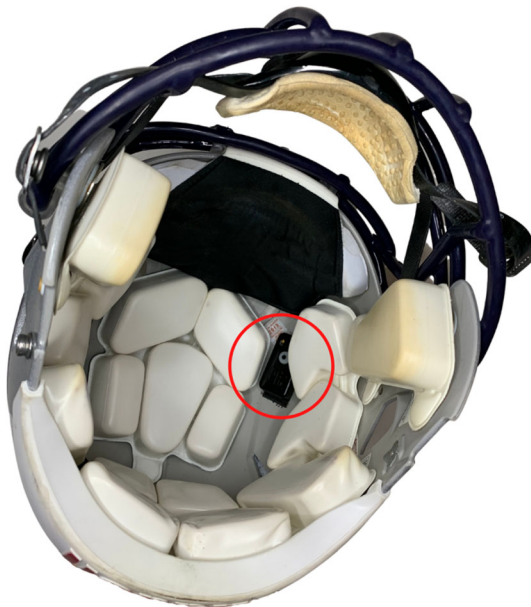
FIGURE 2. GForce Tracker, circled in red, attached to the inside of a Riddell Speed helmet, right of the crown cushion, using an industrial-strength recloseable fastener.
