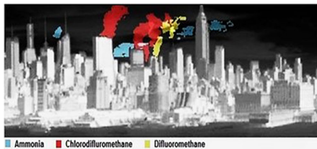
Figure 1. Non-simultaneous composite of compounds detected over Midtown Manhattan. Data cubes post-processed using HyperSEAL software (Aerospace Corp).
