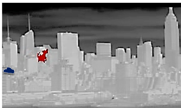
Figure 7. Selected plume for further analysis: (dark red) Chlorodifluoromethane, (dark blue) Ammonia. [Plumes obtained using HyperSEAL software (Aerospace Corp)].
