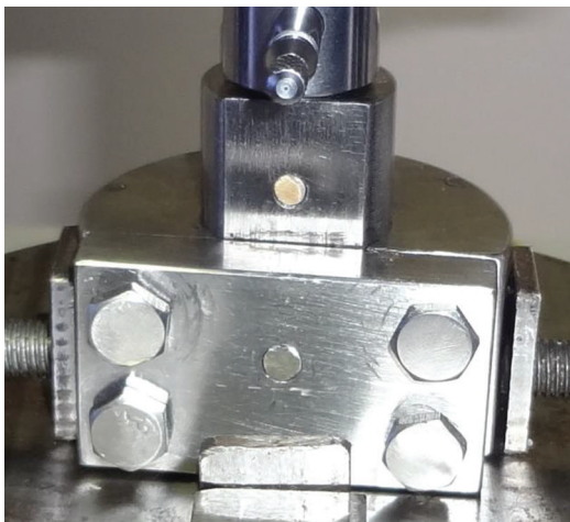
Figure 5: Custom made apparatus mounted in instron for testing samples.
