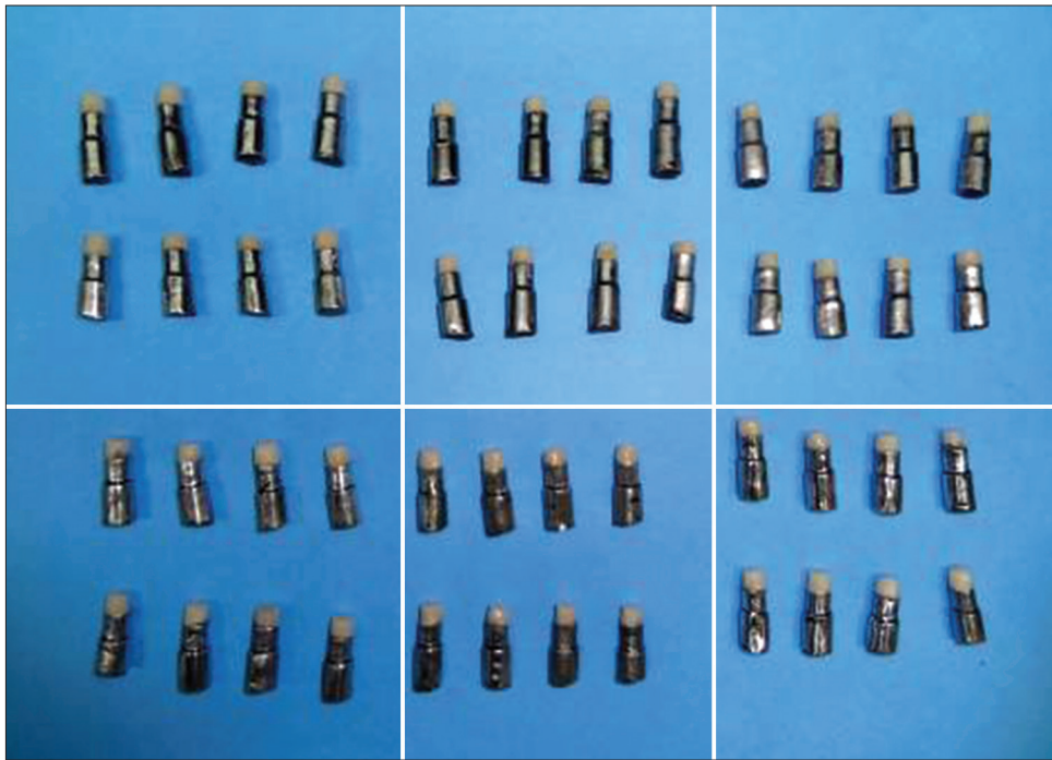
Figure 4: Porcelain firing on the metal samples.
