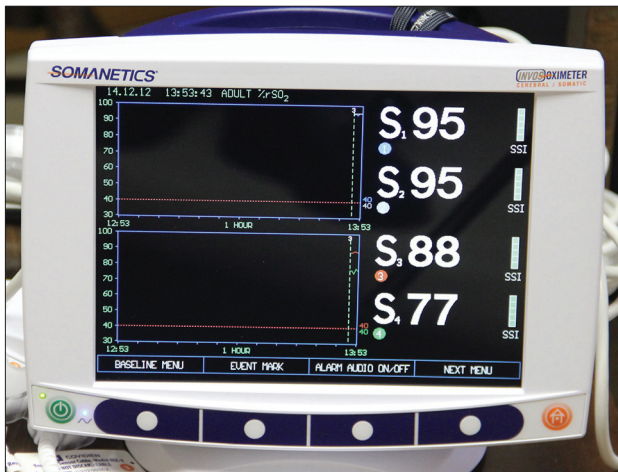
Figure 2: Near-infrared spectroscopy monitor. Equipment for measuring regional oxygen saturation used in this study
