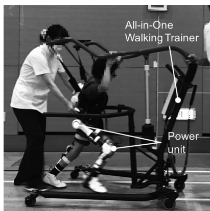
Fig. 1. Gait training using the newly developed smaller Hybrid Assistive Limb with All-in-One Walking Trainer.
