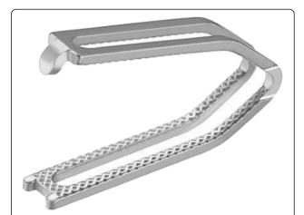
**Fig. 1** DS-Clip. The Aesculap DS Titanium Ligation Clips are made of pure titanium. They are non-ferromagnetic and suitable for MRI. The design of the DS-Clip is characterized by two parallel and interconnected shanks, which prevent axial displacement and clip scissoring. The pyramid-shaped inner surface increases the contact surface of the tissue, ensuring a strong grip
