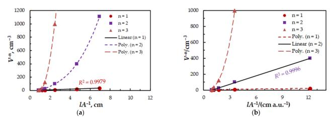
**Figure 6.** Determination of the 4NC:Mo (**a**) and BZC:Mo (**b**) molar ratios by the straight-line method of Asmus. The data are derived from the experimental points in Figure 2.
