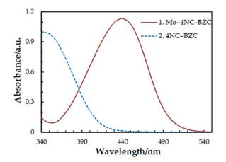
**Figure 1.** Absorption spectra of the complex (1) and blank (2):  $c_{Mo} = 2 \times 10^{-5} \text{ mol dm}^{-3}$ ,  $c_{4NC} = 7.5 \times 10^{-4} \text{ mol dm}^{-3}$ ,  $c_{BZC} = 1.9 \times 10^{-4} \text{ mol dm}^{-3}$ ,  $c_{H2SO4} = 3.75 \times 10^{-2} \text{ mol dm}^{-3}$ ,  $t_{ex} = 3 \text{ min.}$
