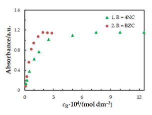
**Figure 2.** Effect of the 4NC (1) and BZC (2) concentration:  $c_{Mo} = 2 \times 10^{-5} \text{ mol dm}^{-3}$ ,  $t_{ex} = 3 \text{ min}$ ,  $\lambda = 439 \text{ nm}$ .  $1-c_{BZC} = 1.9 \times 10^{-4} \text{ mol dm}^{-3}$ ;  $2-c_{4NC} = 7.5 \times 10^{-4} \text{ mol dm}^{-3}$ .
