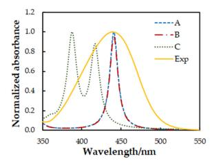
**Figure 8.** Comparison between experimental (Exp) and simulated (A–C) absorption spectra. A Lorentzian broadening and a scaling factor of 0.76 were used for the theoretical spectra.
