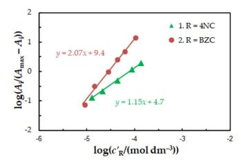
**Figure 5.** Determination of the 4NC:Mo (1) and BZC:Mo (2) molar ratios by the mobile equilibrium method. The data are derived from the experimental points in Figure 2.
