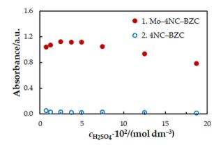
**Figure 3.** Effect of the H<sub>2</sub>SO<sub>4</sub> concentration:  $c_{Mo} = 2 \times 10^{-5} \text{ mol dm}^{-3}$ ,  $c_{4NC} = 7.5 \times 10^{-4} \text{ mol dm}^{-3}$ ,  $c_{BZC} = 1.9 \times 10^{-4} \text{ mol dm}^{-3}$ ,  $t_{ex} = 3 \text{ min}$ ,  $\lambda = 439 \text{ nm}$ .
