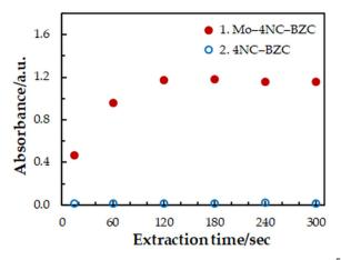
**Figure 4.** Effect of the extraction time:  $c_{Mo} = 2 \times 10^{-5}$  mol dm<sup>-3</sup>,  $c_{4NC} = 7.5 \times 10^{-4}$  mol dm<sup>-3</sup>,  $c_{BZC} = 1.9 \times 10^{-4}$  mol dm<sup>-3</sup>,  $c_{H2SO4} = 3.75 \times 10^{-2}$  mol dm<sup>-3</sup>,  $\lambda = 439$  nm.
