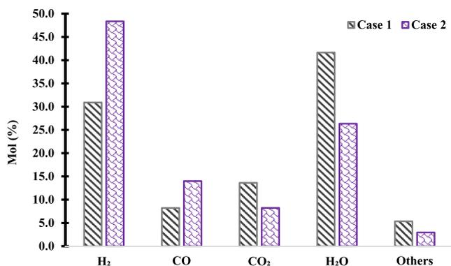
**Figure 4.** Syngas composition for case 1 and case 2.
