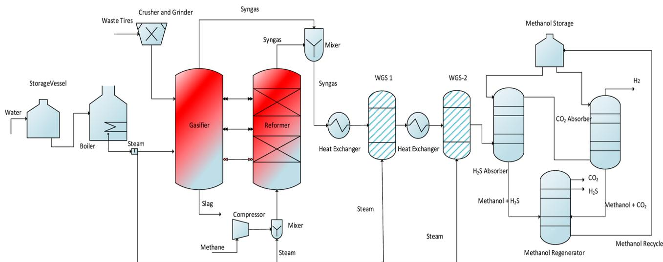
**Figure 3.** Hydrogen production from waste tire gasification and reforming (case 2).
