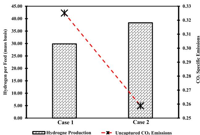
**Figure 6.** Comparison of CO<sub>2</sub>-specific emissions and H<sub>2</sub> production for case 1 and case 2.
