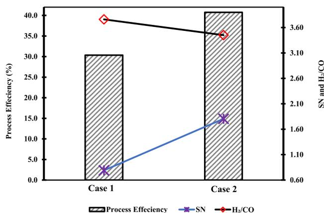
**Figure 5.** Comparison of process efficiency, H<sub>2</sub>/CO, and SN for case 1 and case 2.
