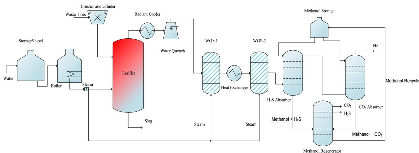
**Figure 1.** Hydrogen production from waste tires (case 1).
