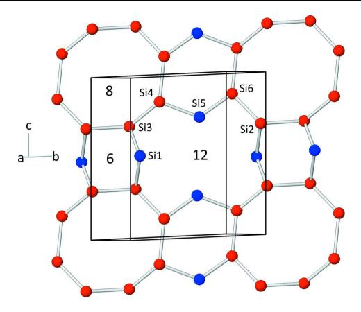
Connectivity of the silicon atoms within a single layer. Red and blue spheres represent  $Q^3$ - and  $Q^2$ -connected atoms, respectively. The sizes of the different ring types are indicated.
