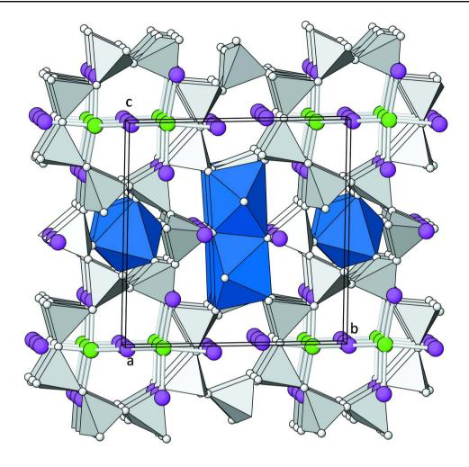
Side view of the whole crystal structure of K<sub>9</sub>Y<sub>3</sub>[Si<sub>12</sub>O<sub>32</sub>]F<sub>2</sub>. [SiO<sub>4</sub>]- and [YO<sub>6</sub>]-polyhedra are shown in light-grey and blue. Small grey spheres represent oxygen atoms. Fluorine and potassium ions are given as larger green and pink spheres. F—K bonds of the  $[F_2K_7]$ -double tetrahedra are indicated.
