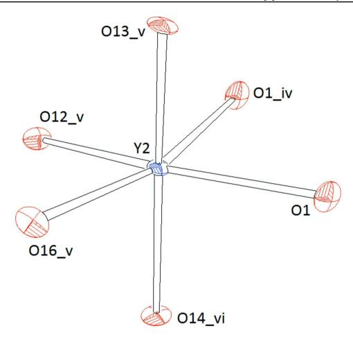
Representation of the coordination polyhedron around Y2. Ellipsoids are drawn at the 60% level. Symmetry codes: [(i) 1 - x,-y, 1 - z; (ii) -1 + x,y,z; (iii) -x,-y,1 - z; (iv) 1 - x,1 - y,1 - z; (v) x,1 + y,z; (vi) 1 + x,1 + y,z; (vii) 1 - x,-y,-z.]
