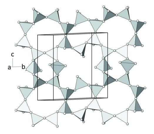
A single silicate layer consisting of [SiO<sub>4</sub>] tetrahedra in a projection perpendicular to (110).
