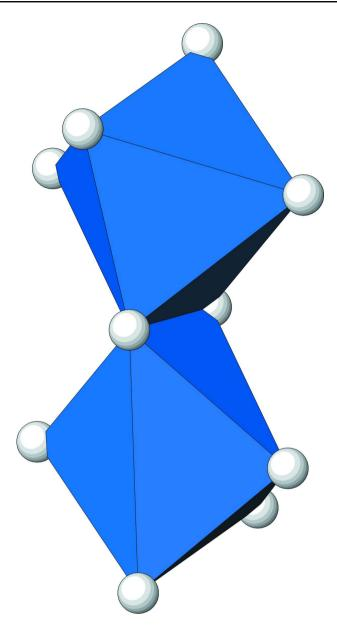
The dimer formed from the condensation of two edge-sharing  $[Y2O_6]$ -octahedra.
