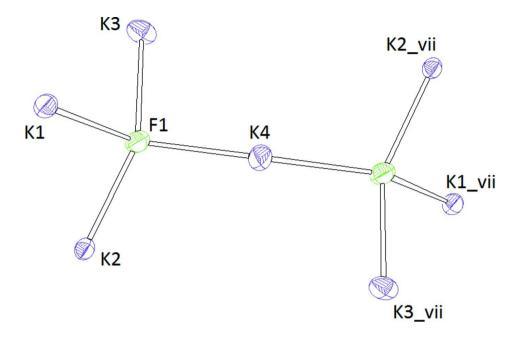
Representation of a single  $[F_2K_7]$ -group. Ellipsoids are drawn at the 60% level. [Symmetry codes: (i) 1 - *x*,-*y*, 1 - *z*; (ii) -1 + *x*,*y*,*z*; (iii) -*x*,-*y*,1 - *z*; (iv) 1 - *x*,1 - *y*,1 - *z*; (v) *x*,1 + *y*,*z*; (vi) 1 + *x*,1 + *y*,*z*; (vii) 1 - *x*,-*y*,-*z*.]
