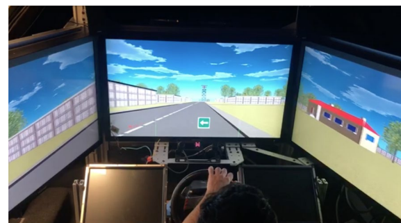
Fig. 1 Driving simulator from the participant's view as they completed the guided navigation phase of the combined landmark group (PD group). Participants controlled their vehicle with a steering wheel, gas, and brake pedals. The small screens on the left and right of the steering wheel were not used in this experiment. In this example, a tall radar tower at the edge of the town (distal landmark), and a colorful house at the upcoming intersection (proximal landmark) are visible to the driver. A white/green navigation arrow briefly presented at the bottom of the central screen indicates a left turn at the next intersection
