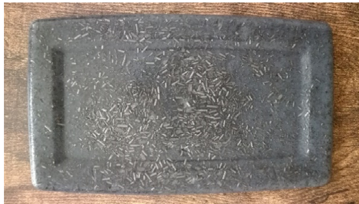
Figure 3. AA phantom simulating a human quadriceps (NaCl concentration = 7 g/L; graphite concentration = 60 g/L).
