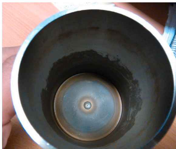
Fig. 12. Liner wear and tear during concurrent grinding inside reactor.
