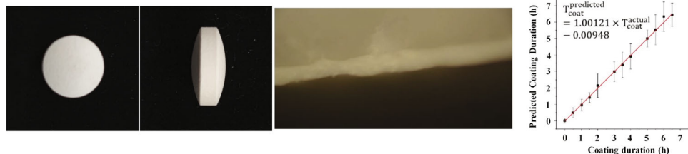
Fig. 6 Detecting the coating thickness of tablets with Raman spectroscopy method [66]. The left figure indicates the optical image of cross-section of the tablet after cleaving and the right diagram indicates the prediction result the drug samples
