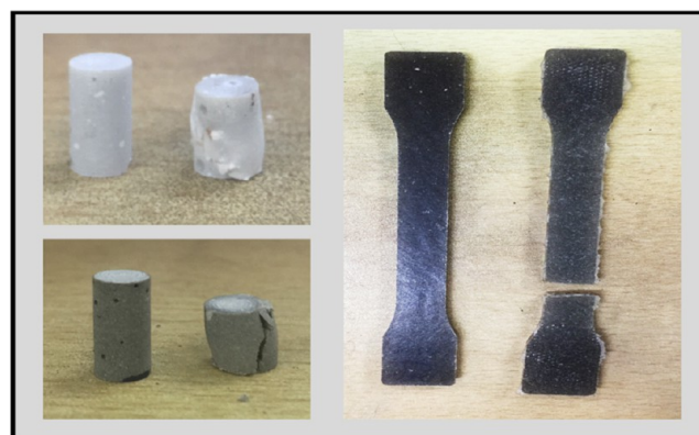
Figure 8. Image of fracture specimens.
