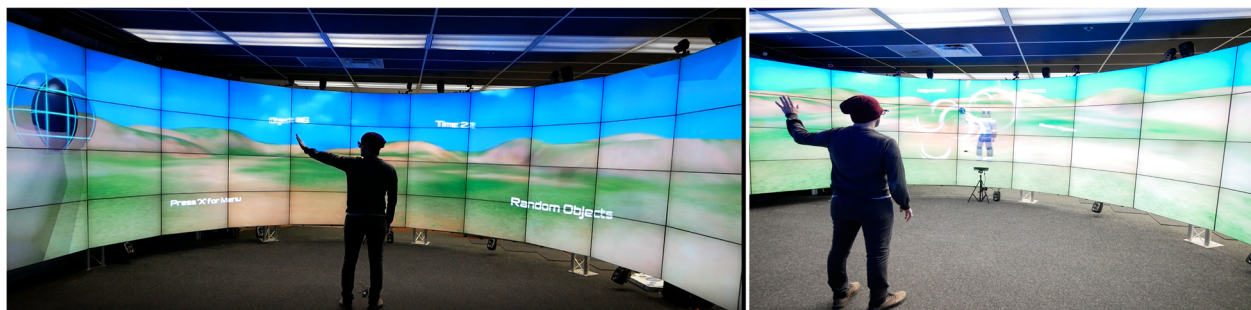
Fig. 8 Rehabilitation application. A nonintrusive immersive application of reaching out and touching stationary objects in space, designed to allow comparison of first-person (left) and third-person (right) perspectives in VR-based rehabilitation
