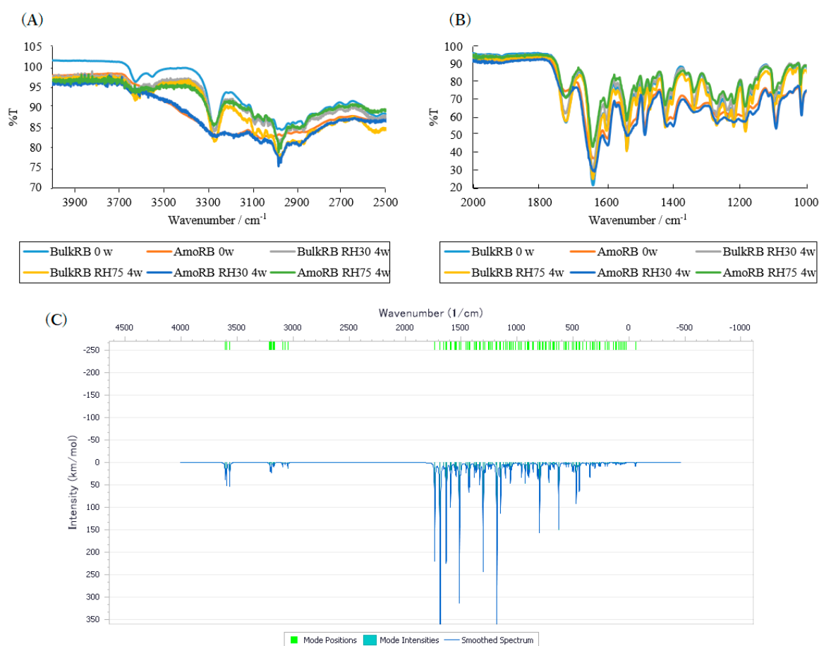
Figure 3. Attenuated total reflection-mid-infrared spectra of RB form I, ground RB and stored samples. RB form I sample stored for 4 weeks in RH 30% and RH 75%. The two regions of 4000 to 2500 cm -1 (A) and 2000 to 1000 cm -1 (B). Simulated IR spectra of RB molecule based on ab initio calculation (C). RH; relative humidity. RB; rebamipide.
