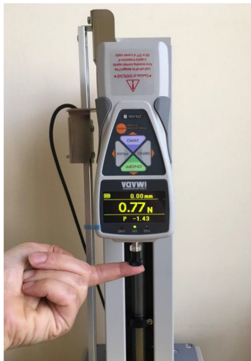
Fig. 9. Force-displacement tests with digital transducer.
