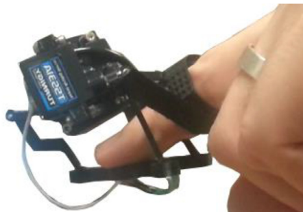
Fig. 1. Example of a wearable haptic device for index fingertip.
