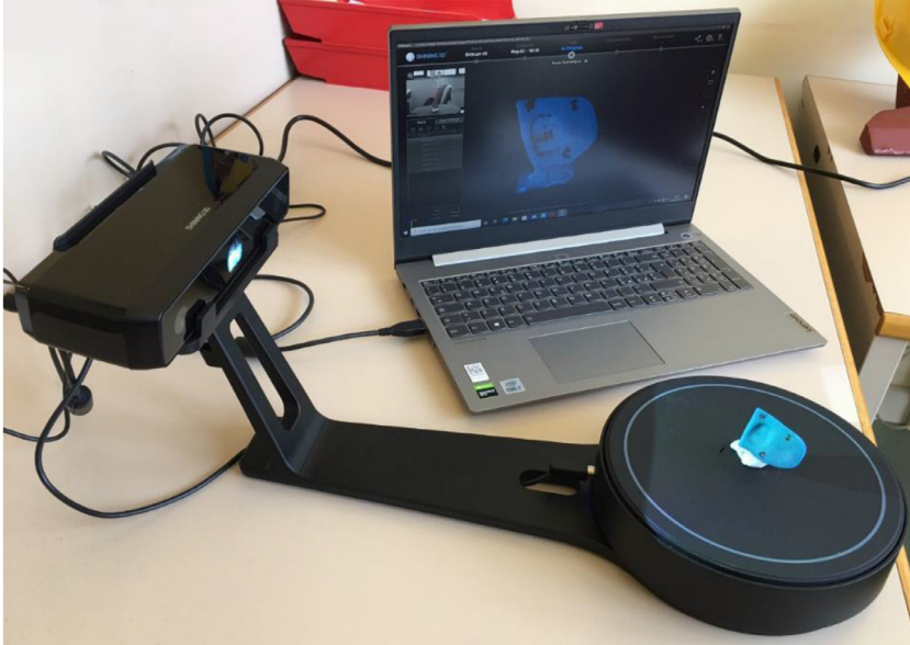
Fig. 12. Impression 3D scanning.
