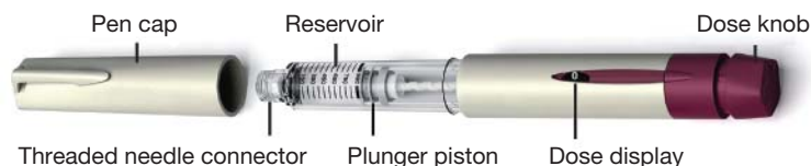
Figure 1. The redesigned follitropin alfa pen injection device.
