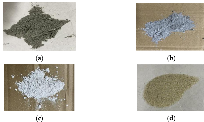
Figure 1. (a) FA, (b) SF, (c) GGBS, and (d) quartz sand used in specimens of this experiment [60].
