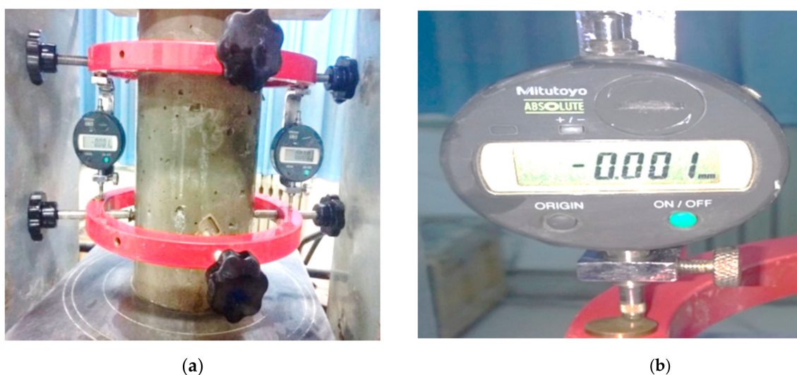
Figure 1. Elastic modulus tester for concrete. (a) Elastic modulus tester; (b) Electronic micrometer measured displacement.
