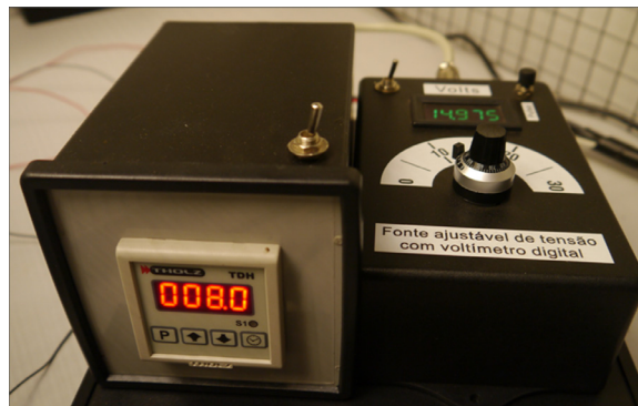
Fig. 3. Adjustable voltage source with digital voltmeter and timer, which allows electrically stimulate plants with certain voltage and duration.
