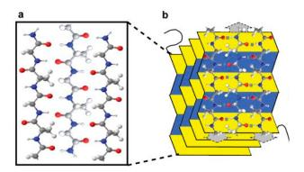
**Figure 10.** An illustration of (**a**) a three chain silk sequence composed of carbon (gray), nitrogen (blue), oxygen (red) and hydrogen (white); (**b**) 3-dimensional  $\beta$ -sheet of silk. Reproduced with permission from [100].
