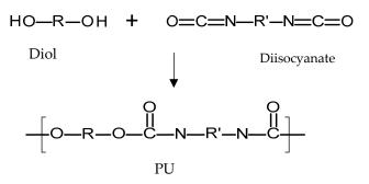
**Figure 7.** An illustration of the chemical structure of poly(urethane) (PU).
