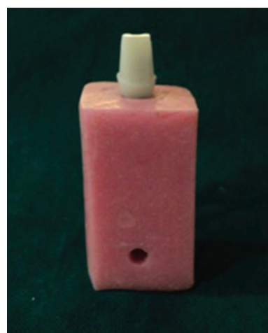
Figure 2: Zirconia abutment mounted on acrylic resin blocks
