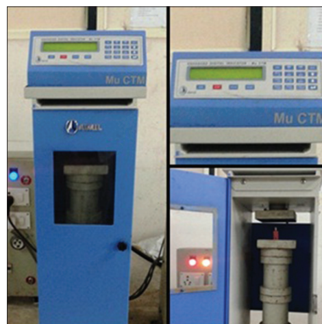
Figure 5: Device used to apply load on coping during cementation
