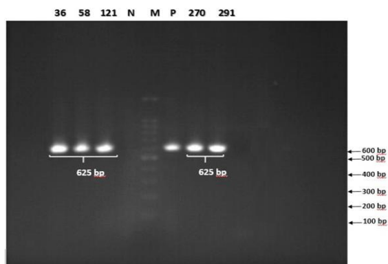
Fig. 2. PCR products for the h7 gene. M: 100 bp DNA ladder, N (Negative control), P (Positive control).
