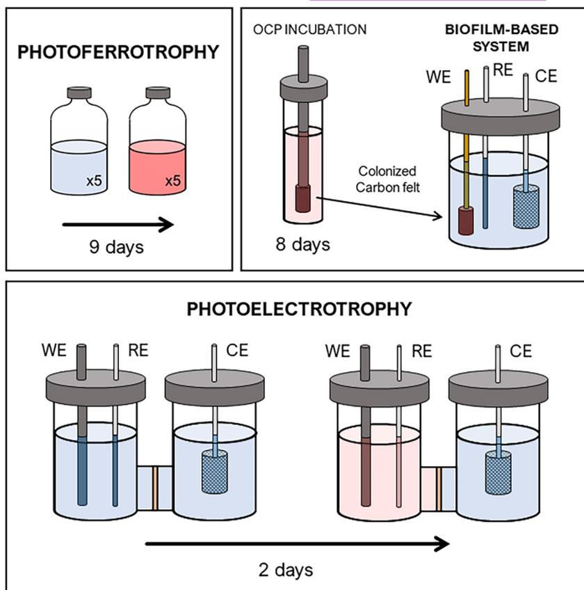
Next, we inoculated H-cell reactor (1/100) with the same inoculum and we operated the reactor at  $-0.6$  V (vs. Ag/AgCl). During growth, we measured absorbance (590 nm) by spectrophotometer and organic compounds by HPLC. At the end of the experiment we visualized the biomass produced by transmission electron microscopy and we analysed microbial population (16S Illumina) at the end of the experiment.
