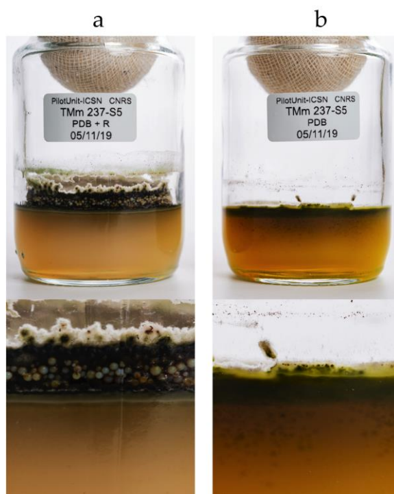
Figure 4. 10 days culture of Chrysosporium lobatum TM-237-S5 on PDA coupled to SSE with XAD TM 16HP N (a) and the control culture on PDA without resin (b). Without the resin (b), the colored compounds were spread in the agar, and their extraction was difficult. With the resin (a), the agar remained clear as the resin beads trapped all the colored target compounds.
