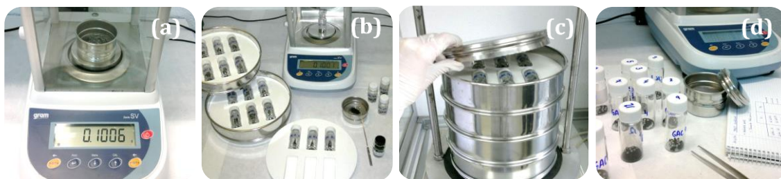
Figure 2. Depiction of materials and procedure for the mechanical strength evaluation of the samples: (a) a weighted sample was sieved using in 300 \mu\text{m} sieve and put in a vial; (b) 15 steel balls were also incorporated in the vial, which was then placed in a polymer mold; (c) the molds were placed in the sieve shaker during 20 min; (d) the sample was sieved again in a 300 \mu\text{m} sieve and the residue (the sample not converted to dust in the sieving step) was collected and weighed to calculate the sample remaining mass percentage (SRM%).
