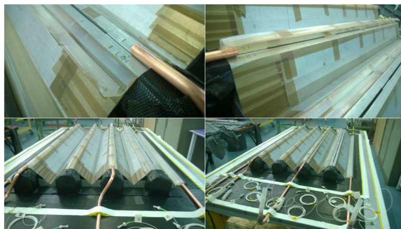
Figure 10. Stringer sensorization with \Omega_{OUT} opened.
