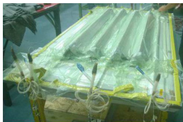
Figure 11. Final panel with sealed vacuum bag, ready for the infusion.
