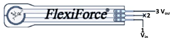
Figure 5. Resistive sensor FlexiForce A201 ® connection diagram, where node 1 refers to input voltage, and node 2 refers to ground and node 3 refers to output voltage.
