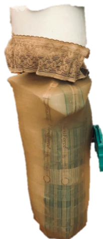
Figure 12. Artificial residuum with the socket interface pressure (SIFP) sensor and F-Socket sensors before the socket is installed.
