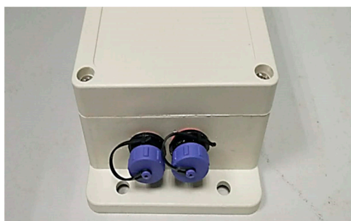
Figure 3. Plug perforated on the side of the device box.
