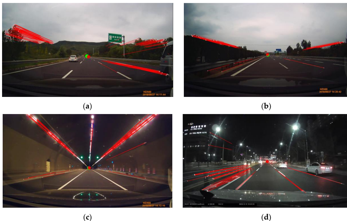
Figure 7. Some examples of the proposed motion-based R-VP detection in various illumination conditions such as (a) bright and (b) slightly dark daytime, (c) tunnel, and (d) nighttime. Note that ground-truth R-VP is not indicated in (d).
