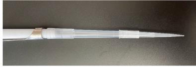
**Figure 4. P1000/P200 pipette tip stacking for careful aspiration following urea washes**
