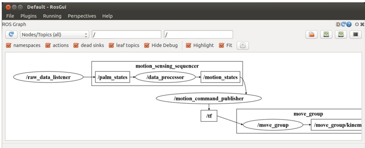
Fig. 8 Nodes and topics in motion sensing layer. The sequencer subscribes raw sensor data published by sensor driver, then performs data processing and publishes captured motion states
