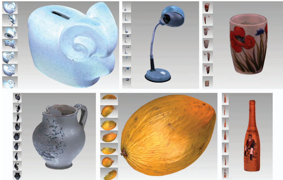
Figure 1. Examples of 3D model acquisition and registration. For each presented object, the insets on the left show the different 3D raw scans used to build the complete object model.
