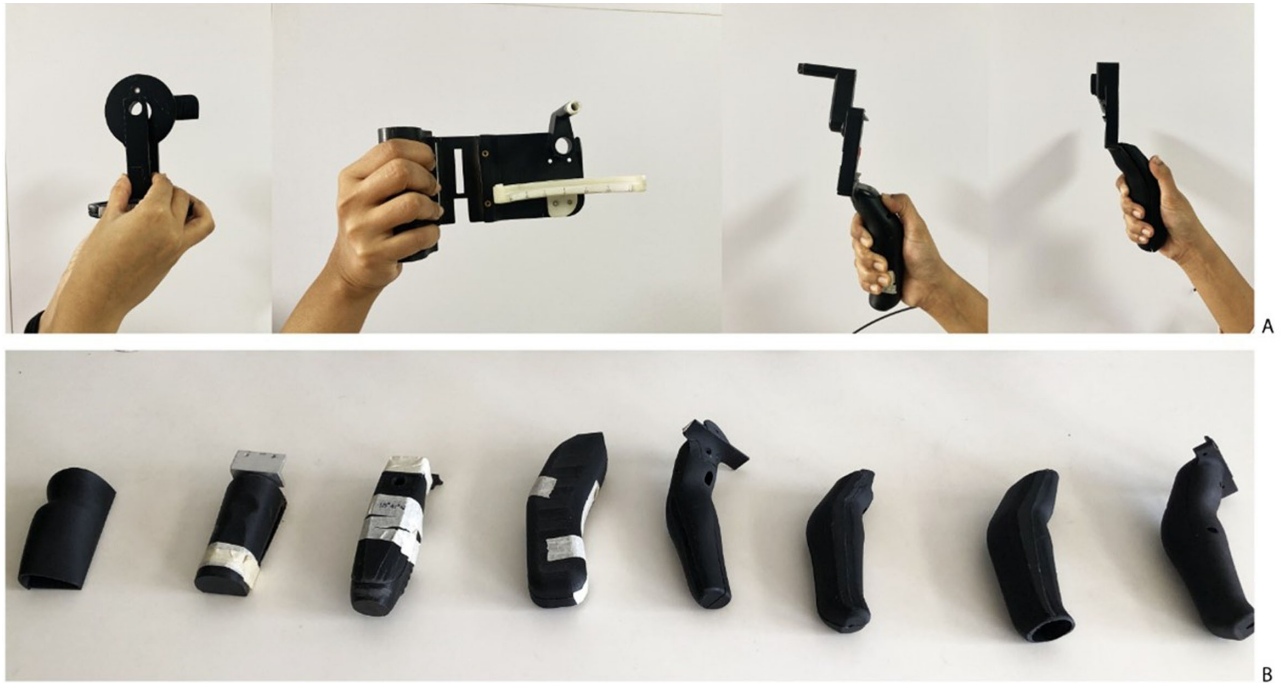
Figure 2. (A) The initial prototypes for the PSL D20 designed based on ease of handling. From a design that required both hands for operation, we deduced a design which was suitable for one-handed use. (B) A line of handles prototyped for ease of use for the PSL.
