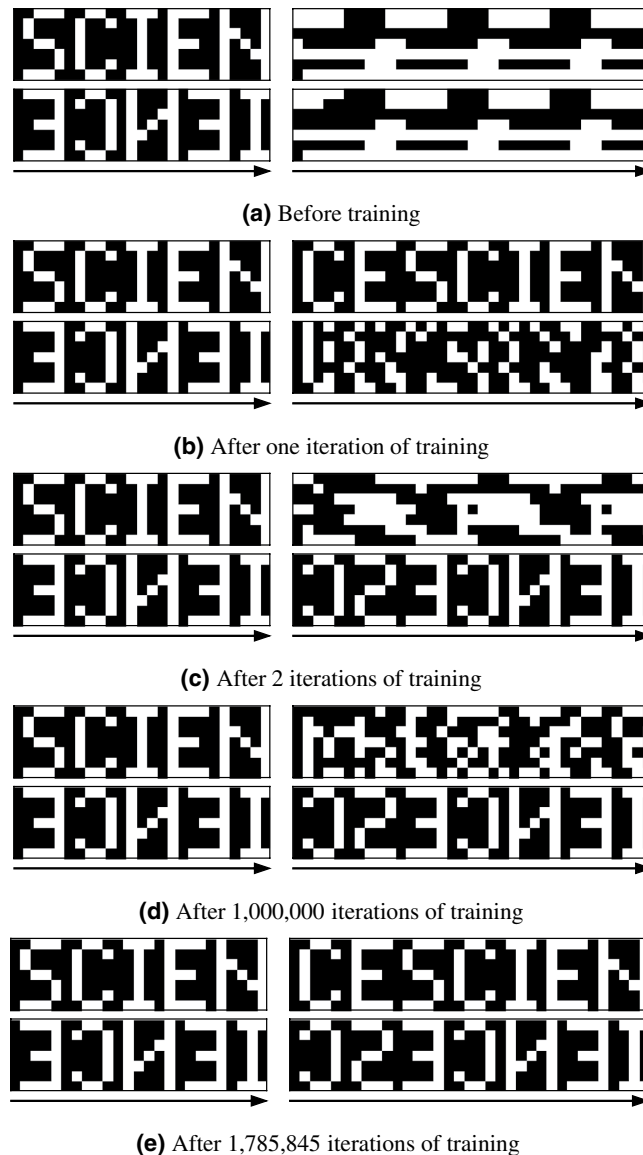
Figure 5. The DyBM learned two target sequences and retrieved a particular sequence when an associated cue was presented. The DyBM generated the right sequence after the left sequence was presented as a cue. (a) The DyBM did not generate the target sequences prior to training. (b) The DyBM learned the first target sequence “SCIENCE” in the first iteration and retrieved it when its partial sequence was presented as a cue. (c) After the second iteration, the DyBM retrieved the second target sequence of the mirror image of “SCIENCE” but not the first. (d) After one million iterations, the DyBM learned the second target sequence, while keeping a partial memory of the first. (e) The DyBM eventually retrieved one of the two target sequences, depending on the cue.
