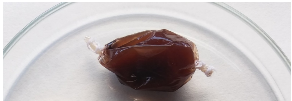
Fig 1. Semipermeable cellulose membrane capsule containing 30 mg of biosorbent per mL of deionized water (EB30).
