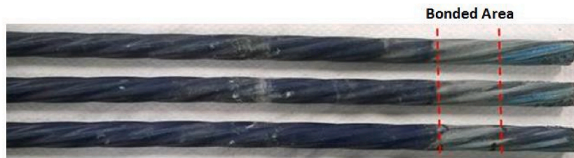
Fig. 18. Visual appearances of the pulled-out prestressing strands with the hybrid epoxy coating applied via electrostatic spray to individual wires in the course of their helical winding into seven-wire strand.
