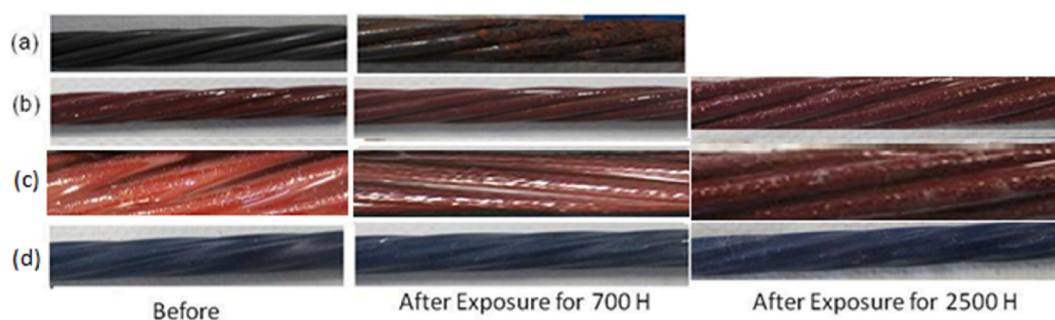
Fig. 12. Views of prestressing strands coated with various epoxy systems before and after 1 month of exposure to salt fog spray: (a) bare strand; (b) self-heal epoxy; and (c) self-heal toughened -I epoxy; and (d) hybrid (self-heal/nanocomposite/toughened) epoxy.
