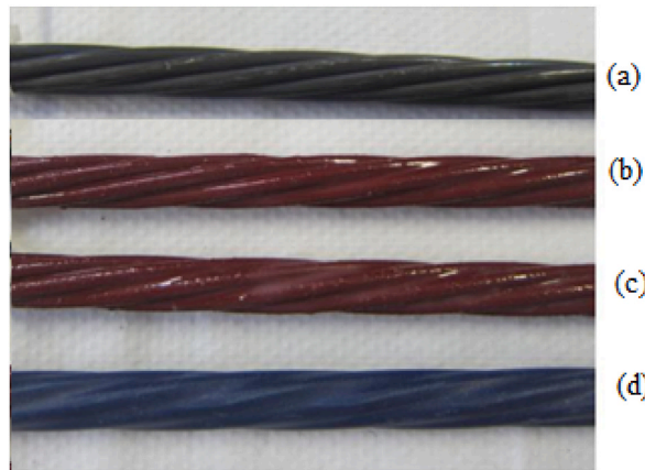
Fig. 2. Photographs of prestressing strands: (a) uncoated; (b) self-healing epoxy (c) self-healing/toughened epoxy-I; and (d) hybrid self-healing epoxy.
