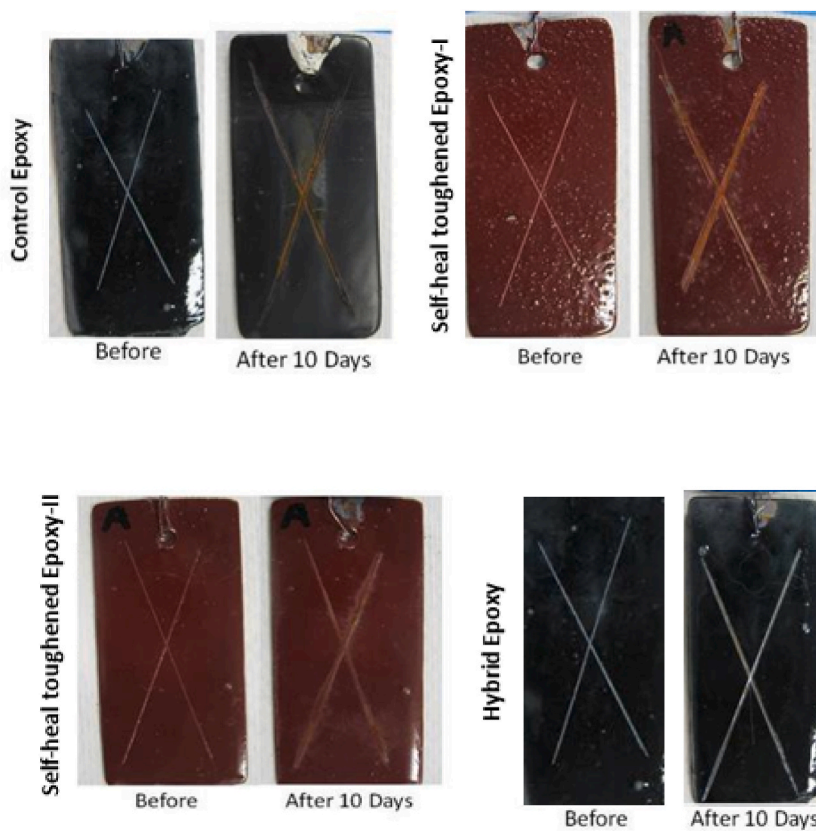
Fig. 16. Scratched surfaces of steel plates with different epoxy coatings before and after exposure to 3.5 % NaCl solution for 10 days.
