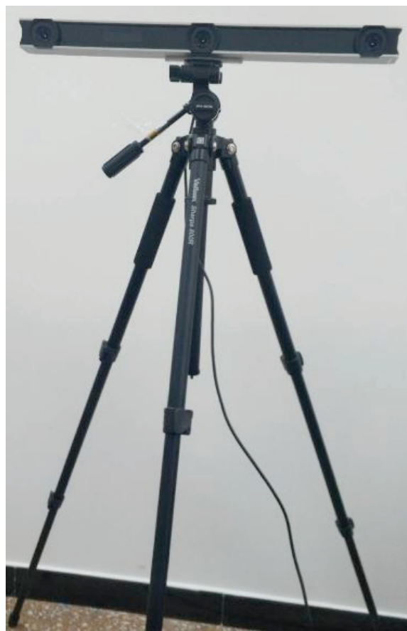
Figure 2. OptiTrack-V120: Trio device which represents the optical motion capture system. The device was fixed with a 3-foot frame to ensure that the three cameras were placed in a horizontal position.
