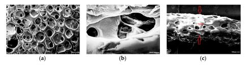
**Figure 5.** SEM micrographs of MPTL scaffold: (a) surface  $\times 100$ ; (b) scaffold interior  $\times 10,000$ ; and (c) scaffold thickness  $\times 100$  times.
