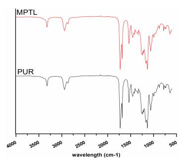
Figure 2. FTIR spectra of PUR and MPTL scaffolds.
