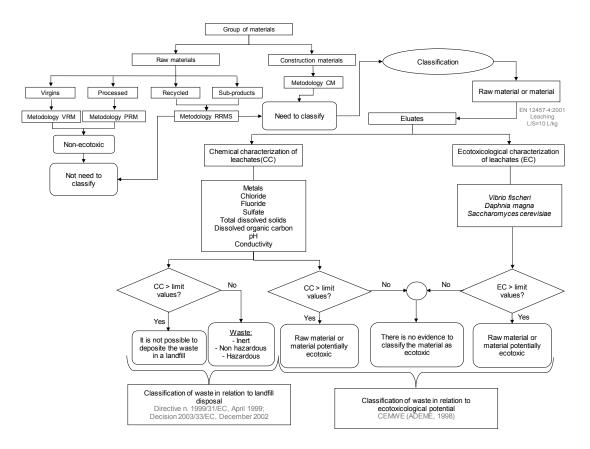
**Figure 2.** Flowchart representing the methodology for the performance of the chemical and ecotoxicological characterization, and classification of raw and construction materials.
