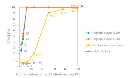
**Figure 5.** Effect (% of control) on the test organisms when exposed to different concentrations of the A1 eluate sample.
