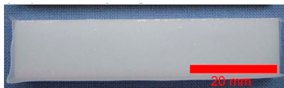
Figure 2. GUR molds after pressing, red bar = 20 mm.
