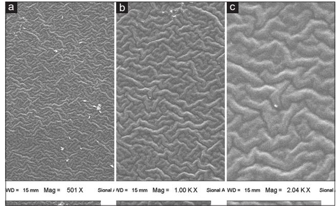
**Figure 2:** Scanning electron microscope (SEM) photographs of the anterior surface showing undulated “maze” pattern surface degradation at a magnification of (a) 501 × (b) 1000 × and (c) 2000 ×
