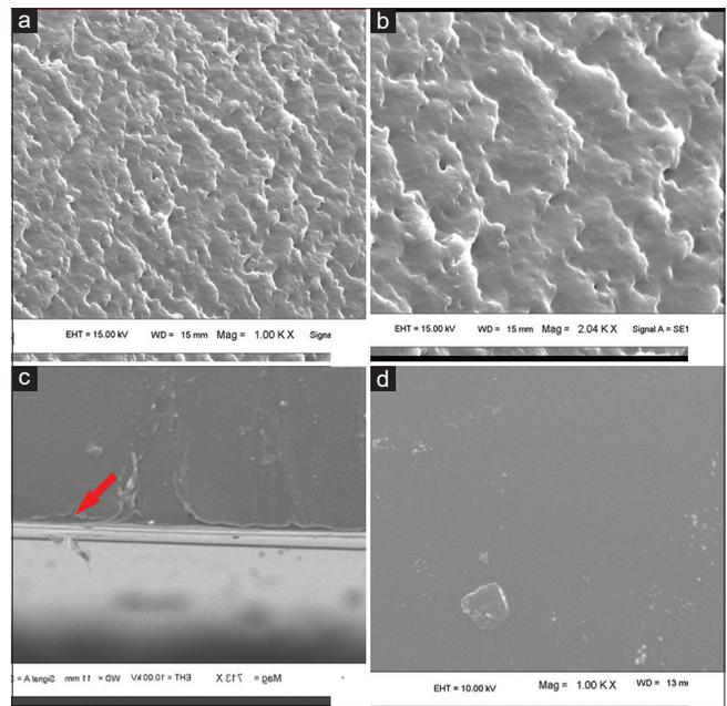
**Figure 4:** Magic coral pattern and microvacuoles of various sizes throughout the thickness of the IOL optics at a magnification of (a) 1000 × and (b) 2000 × and (c) Loss of contact between the posterior lens capsule and IOL surface (red arrow). (d) No patterns of degradation in the cut-section of the control specimen
