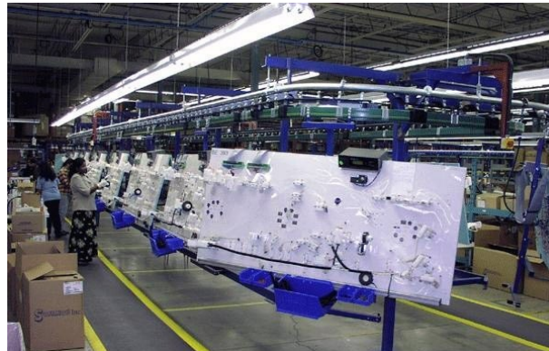
Figure 1. The wire harness paced assembly conveyor (often referred to as a rotary) contains assembly tables consisting of connector and clip fixtures [18].
