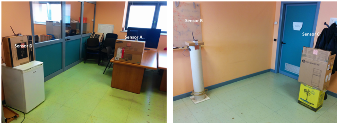
Figure 7. Sensor A, B, C and D placement in the experiment room.
